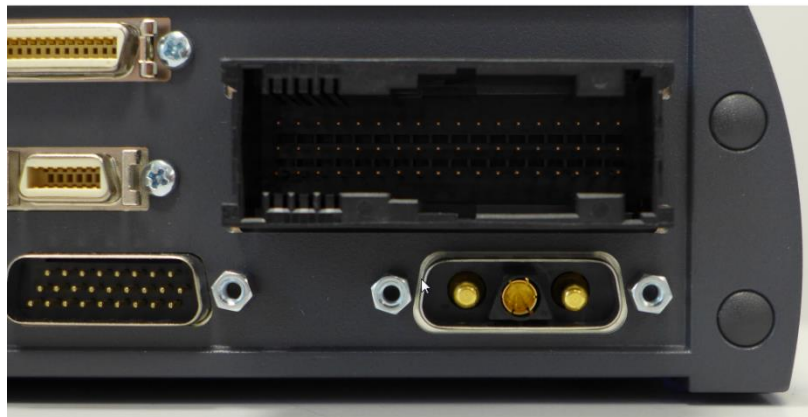
Figure 7.11: new power supply connector with reverse polarity protection
