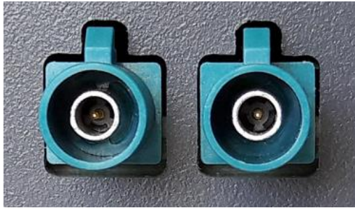
Figure 14.10: MOST150 cPhy Connector, electrical Simplex / Duplex
