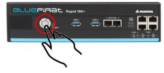
To switch off the BLUEPIRAT Rapid later, please press the **[ON / Trigger]** button for a few seconds, until the green LED starts pulsing.
