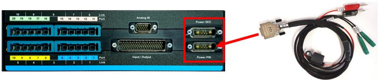
Figure 9.1: BLUEPIRAT Rapid – connecting the power supply
