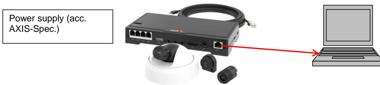
Figure 5.1 Connecting the network camera with a PC/ laptop
