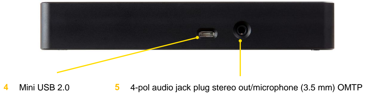
Figure 5.3: Rear side view with components
