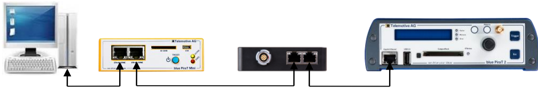
Figure 5.5: TSL network with one bPMini, one Remote Control Touch and one bP2 (e.g.)
