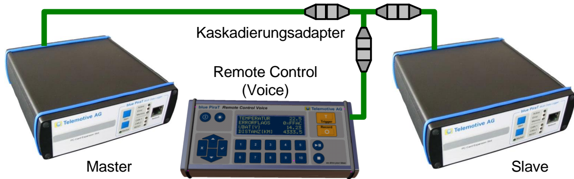
Figure 5.2: Connecting the RCV adapter with cascading
