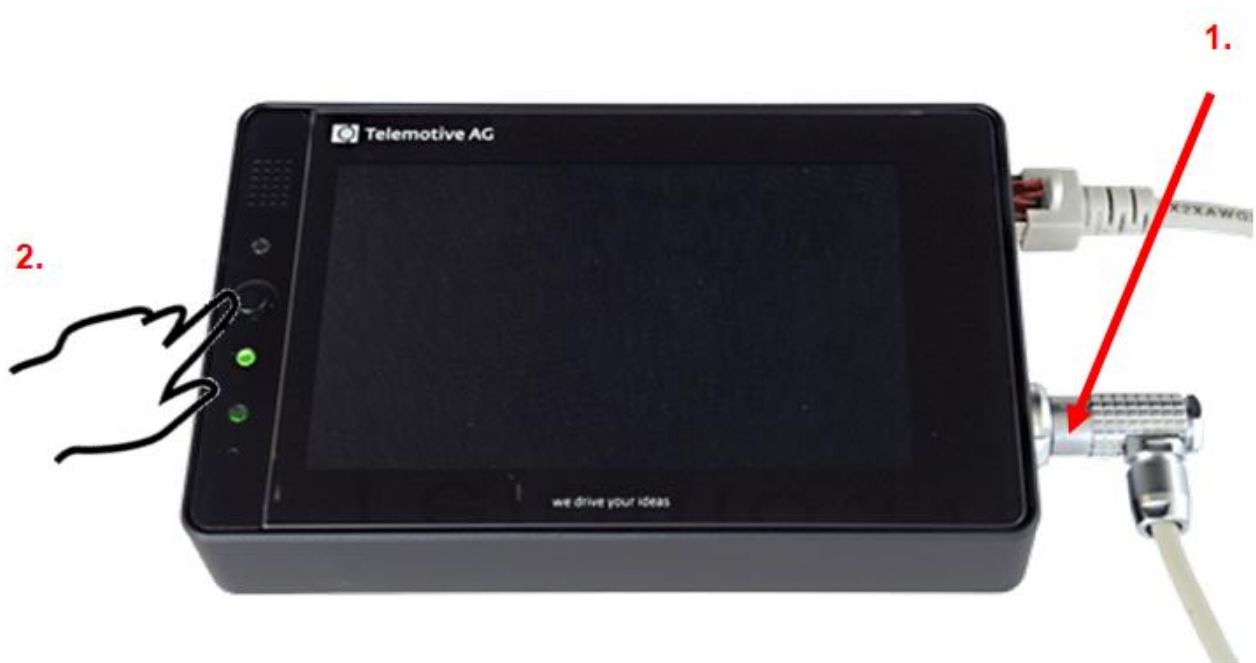
Figure 5.7: Switching on the Remote Control Touch
