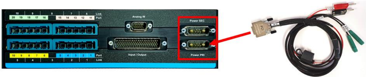
Figure 5.2: BLUEPIRAT Rapid – connecting the power supply
