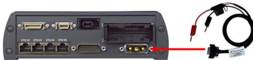
Figure 5.9: Power connection on the BLUEPIRAT2 5E
