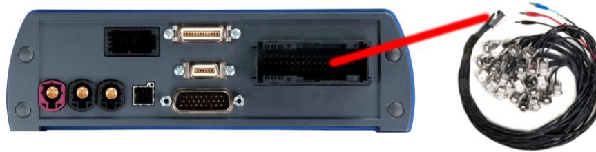
Figure 5.8: Power connection on the BLUEPIRAT2
