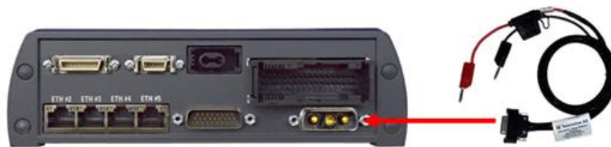
Figure 5.2: Power connection on the blue PiraT2 5E
