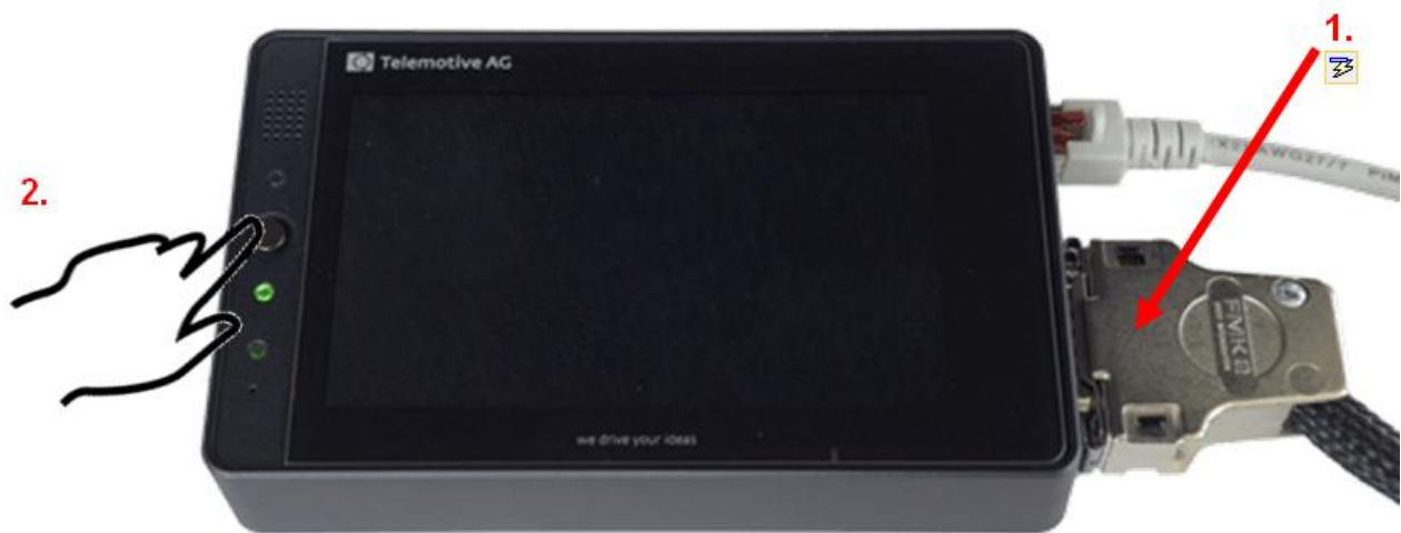
Figure 5.7: Switching on the blue PiraT Remote
