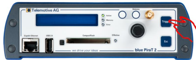
Figure 5.3: Switching on the blue PiraT2
