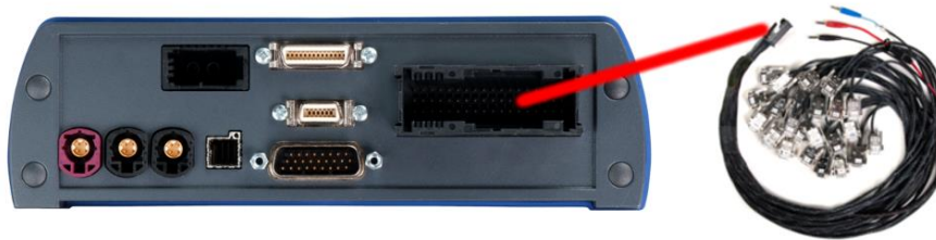
Figure 5.1: Power connection on the blue PiraT2
