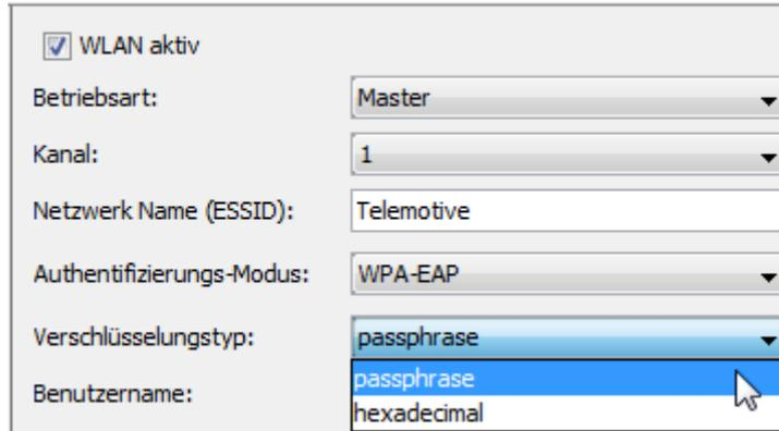
The screenshot shows a configuration window for WLAN. The 'WLAN aktiv' checkbox is checked. The 'Betriebsart' is set to 'Master', 'Kanal' to '1', and 'Netzwerk Name (ESSID)' to 'Telemotive'. The 'Authentifizierungs-Modus' is 'WPA-EAP'. The 'Verschlüsselungstyp' dropdown menu is open, showing 'passphrase' selected and 'hexadecimal' as an alternative option. The 'Benutzername' field is empty.
