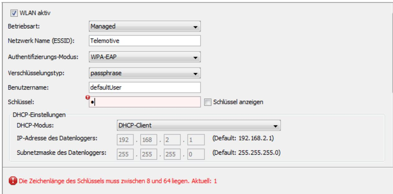
The screenshot shows the same configuration window as in 5.18, but now with a key entered in the 'Schlüssel' field. A red warning icon and message are visible: 'Die Zeichenlänge des Schlüssels muss zwischen 8 und 64 liegen. Aktuell: 1'. The 'Schlüssel anzeigen' checkbox is unchecked. Below the key field, the 'DHCP-Einstellungen' section is visible, with 'DHCP-Modus' set to 'DHCP-Client', IP address '192.168.2.1', and subnet mask '255.255.255.0'.
