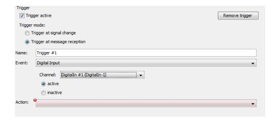
The condition "active" is true, when the voltage level of the digital input correspond to the chassis ground (KL31).
