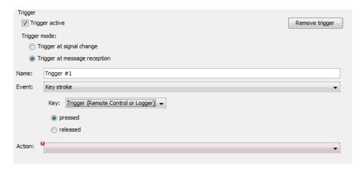
The related action is executed once when the event condition key "pressed" or key "released" changes into the status "true". A connected blue PiraT remote control is required for an event with a function key.
