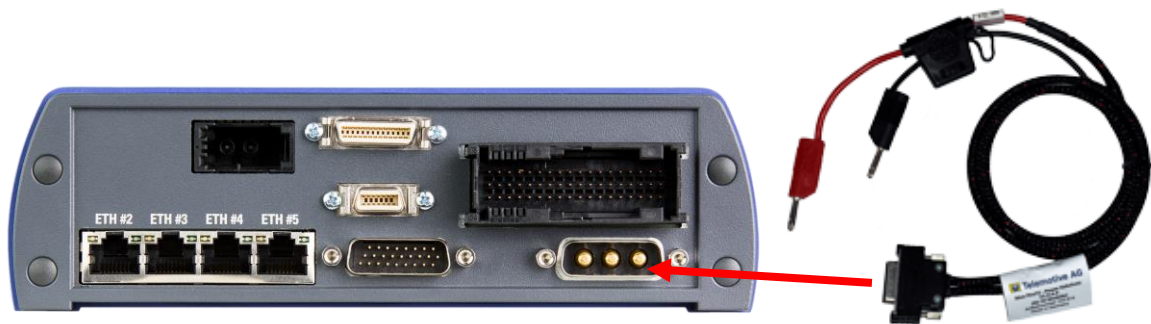
Figure 7.2: Power connection of the blue PiraT2 5E
