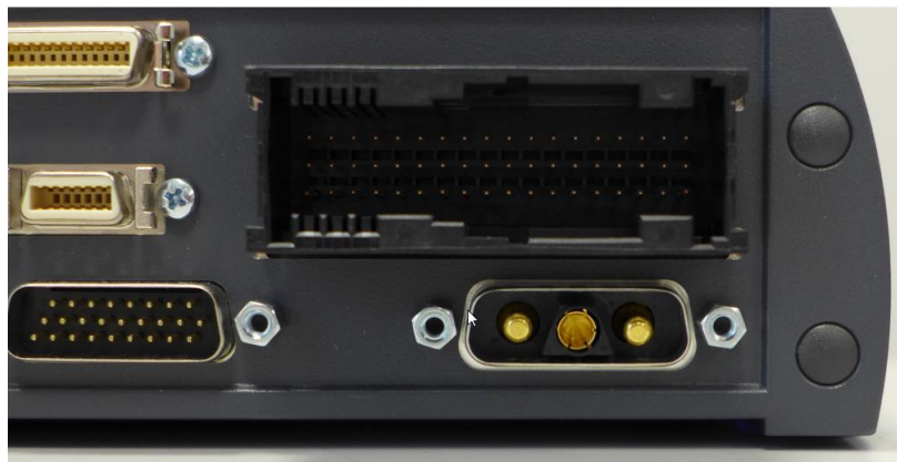
Figure 7.10: new power supply connector with reverse polarity protection
