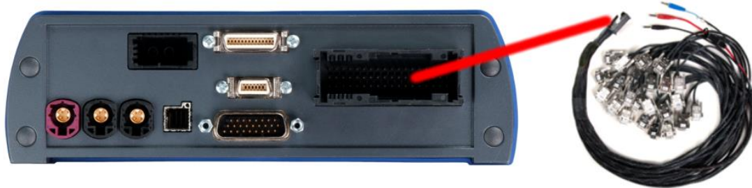
Figure 7.1: Power connection of the blue PiraT2
