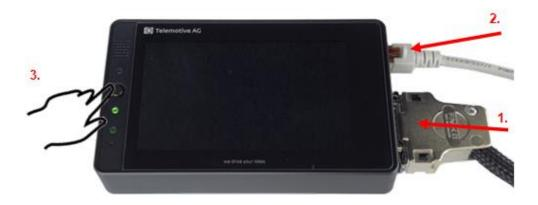
**Step 2:** Connect one Ethernet port with the Ethernet port of your computer by using a Ethernet cable. **(2.)**
